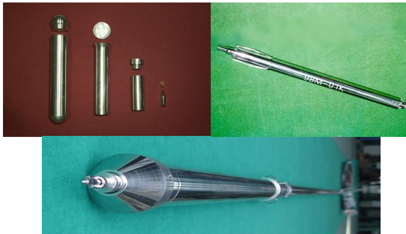
Fig. 2. Irradiation rabbit, non-instrumented capsule and an instrumented capsule.
